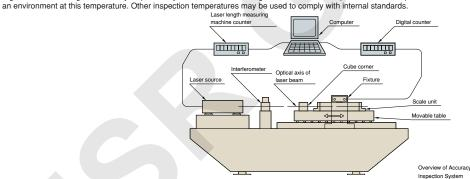
The accuracy of the scale at each point is defined in terms of an error value that is calculated using the following formula: Error = Value indicated by laser inspection system — Corresponding value indicated by the linear scale
